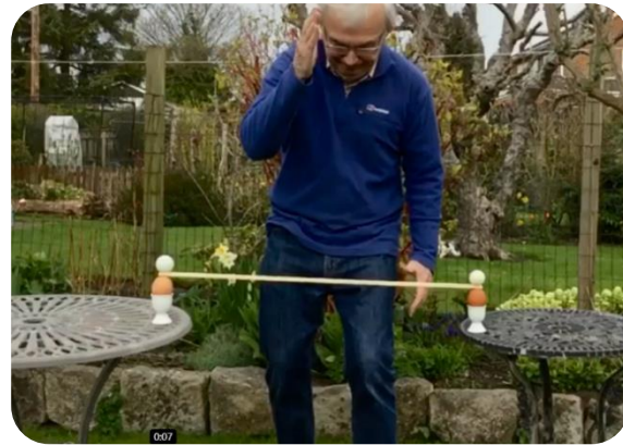
Figure 2: The modified set up with two fresh eggs as supports for the rod. Table tennis balls are balanced on the rod above the eggs in order to show the resultant motion.
