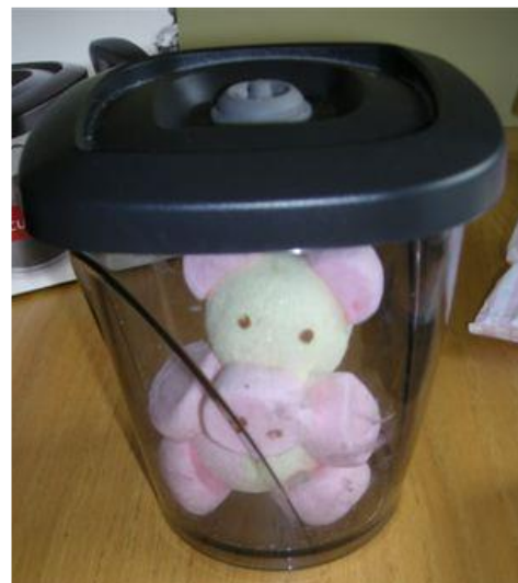
Low pressure, marshmallows have expanded
