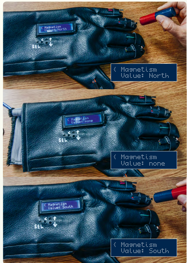
@ 1a-c: Determining the poles of a magnet
